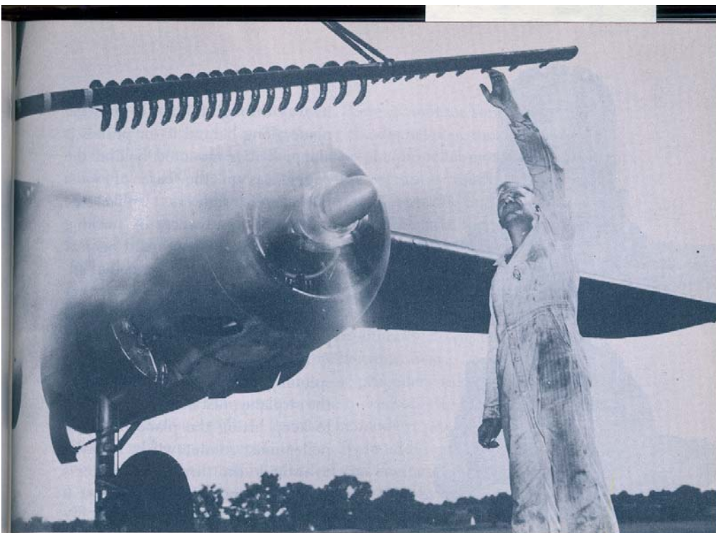
The nozzles in this testing device spray the propellers with water. At 20,000 feet ice forms, to permit engineers to test the value of de-icing equipment.
