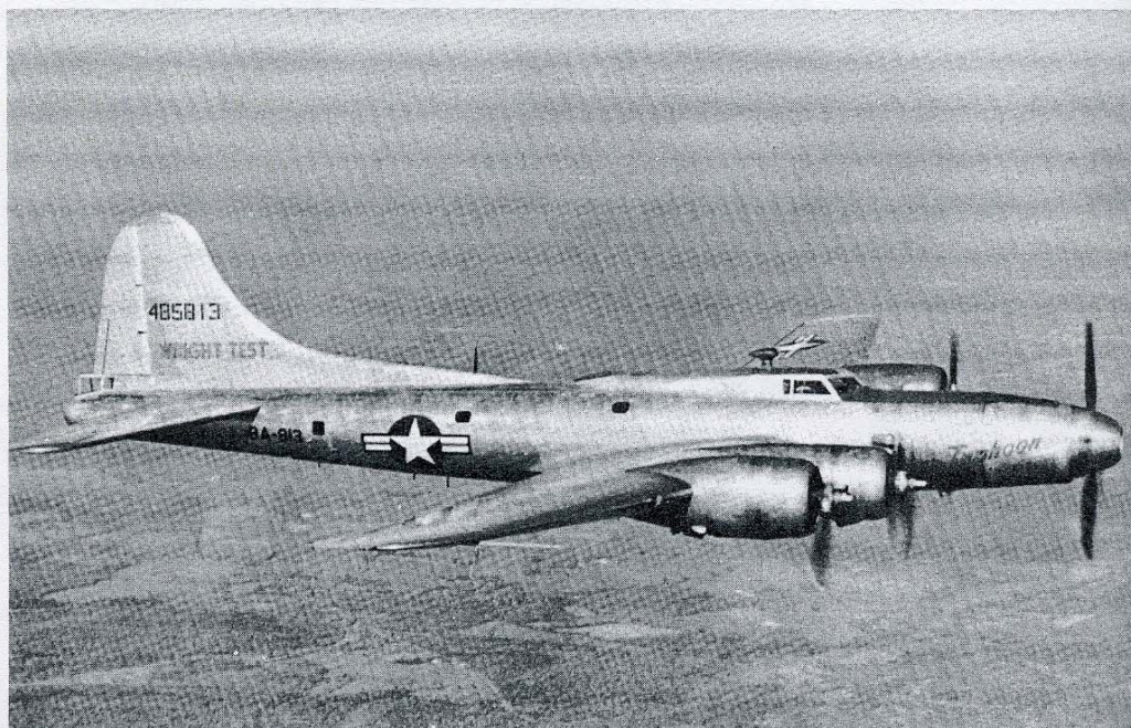
This is Wright's flying laboratory for turbines. Engines and propellers are installed in its nose for tests under actual flight conditions.
