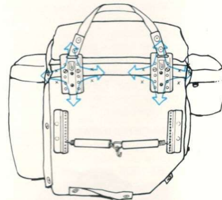
Note the adjustability afforded by this new carrier hook system.
